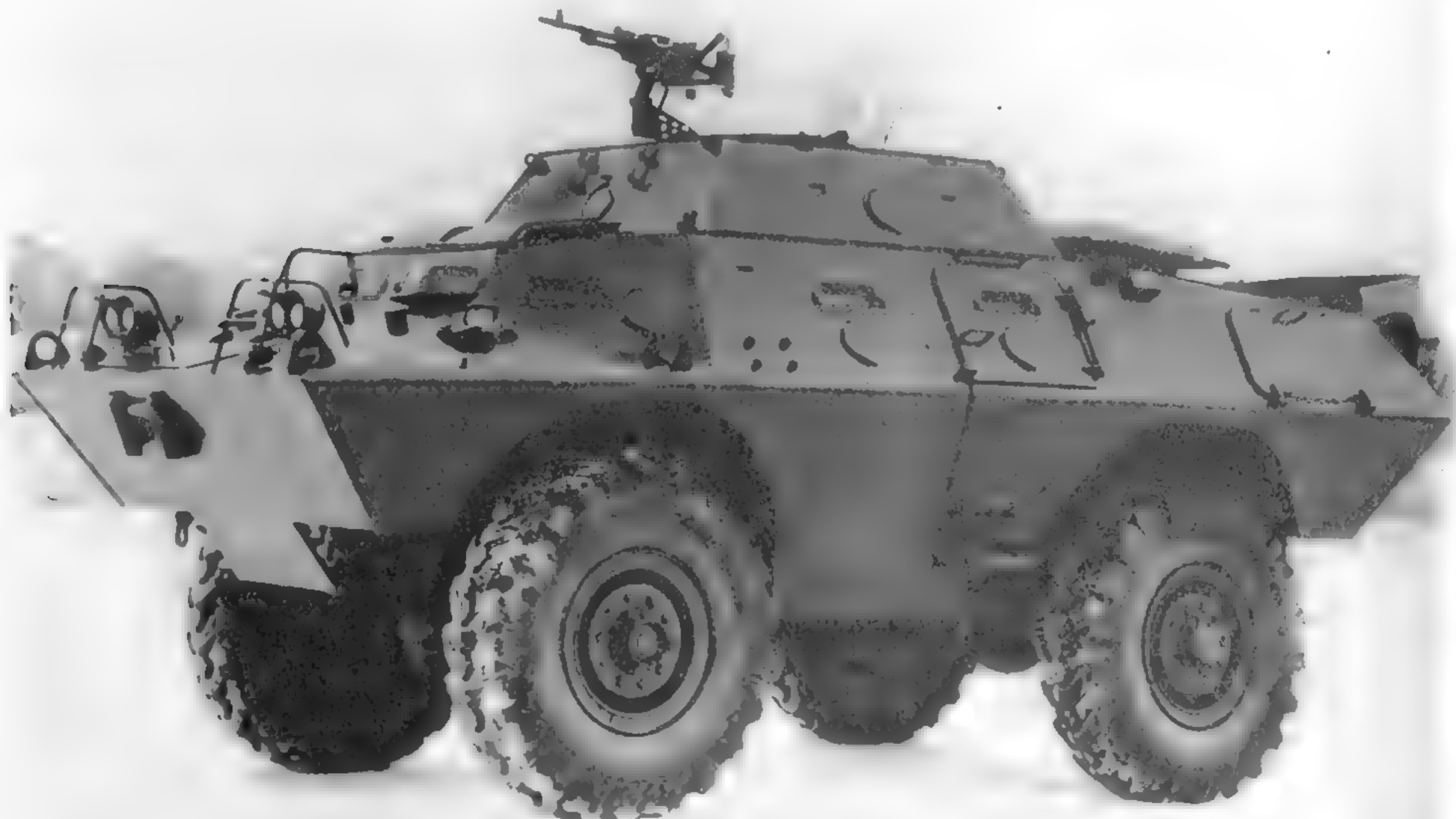
The XM706E2 lacked the turret of the XM706, instead having an open-top compartment on the roof. The XM706E2 was the version of the V-100 that was most popular with the Air Force. (Photo courtesy of the Patton Museum)
